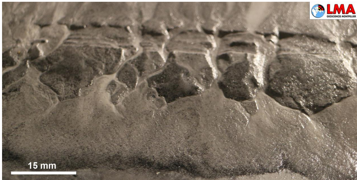
Figure 1 : Detailed view of an analog model surface during a geomorphological experiment including reverse faulting.
